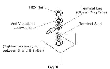
Recommended method of connection to electrical terminals. All terminal hardware, including lug, supplied with unit.
